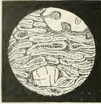
Axiolite.—Specimen of rhyolite from Virginia Range, Nevada, magnified two diameters. (From Zirkel's "Microscopical Petrography.")
